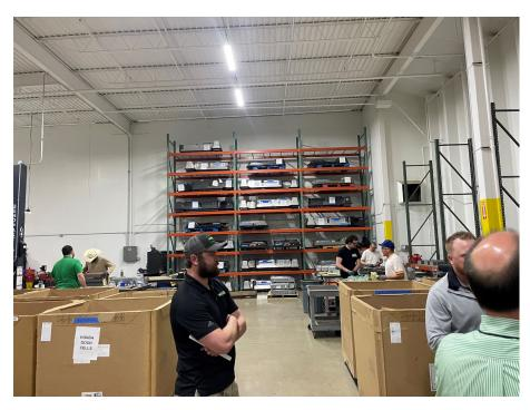
Figure 3. Disassembly, sorting, and testing room; boxes with "good" battery cells, shelving with reassembled batteries.
