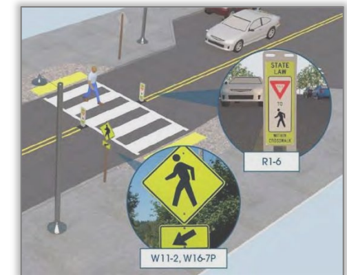
Figure 10 - High-Visibility Crosswalk (FHWA)
