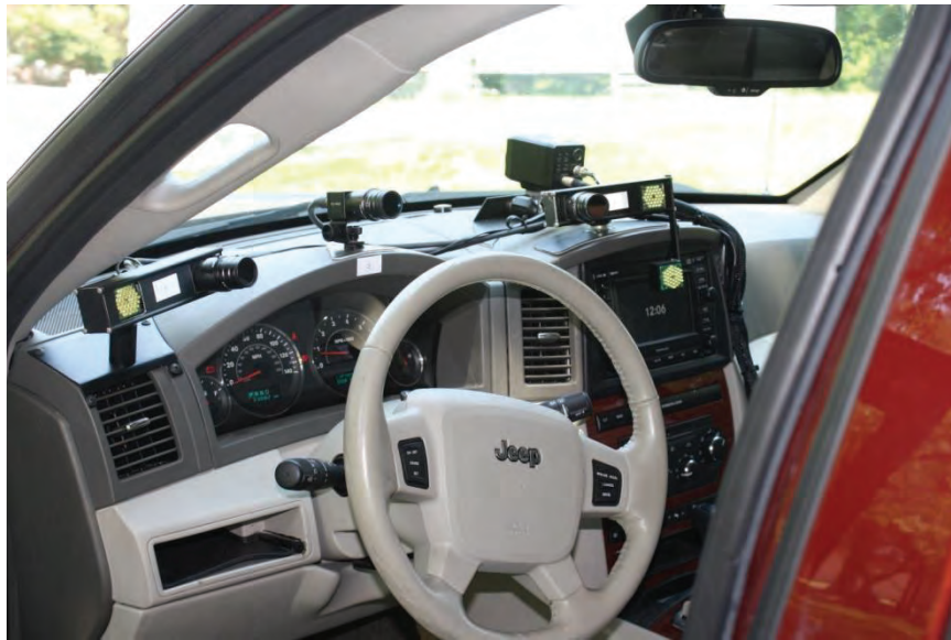
Figure 1. Eye tracking system camera placement.
