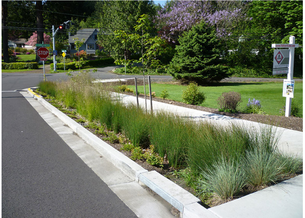
Figure 9.10 - Blue-Green Infrastructure Example
