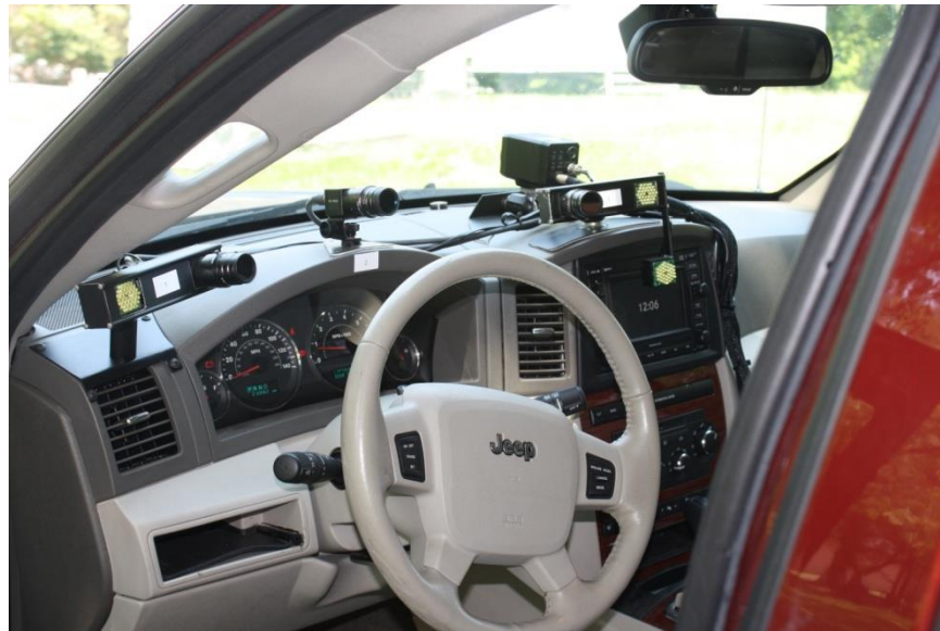
Figure 1. Eye tracking system camera placement.
