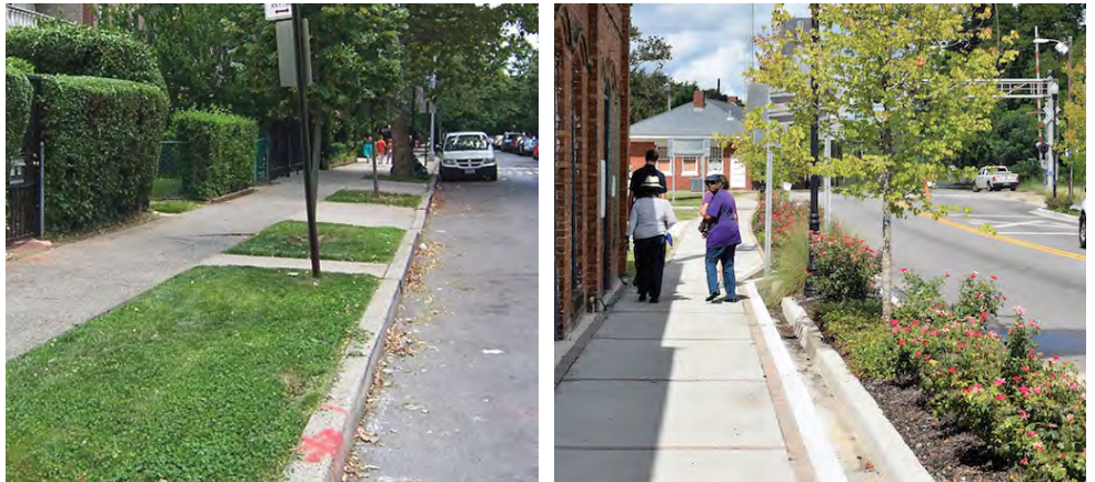
Figure 6.9 - A Vegetated Buffer Creates a Safe and Comfortable Environment for both Pedestrians and Vehicles
