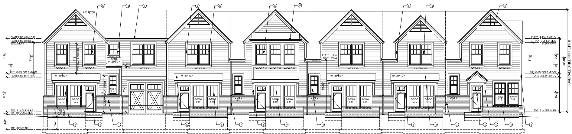
UNIT 17 - B PLAN UNIT 16 - C PLAN UNIT 15 - A PLAN UNIT 14 - A PLAN UNIT 13 - C PLAN UNIT 12 - A END PLAN FRONT - NORTH ELEVATION SCALE - 1/4" = 1'-0"
