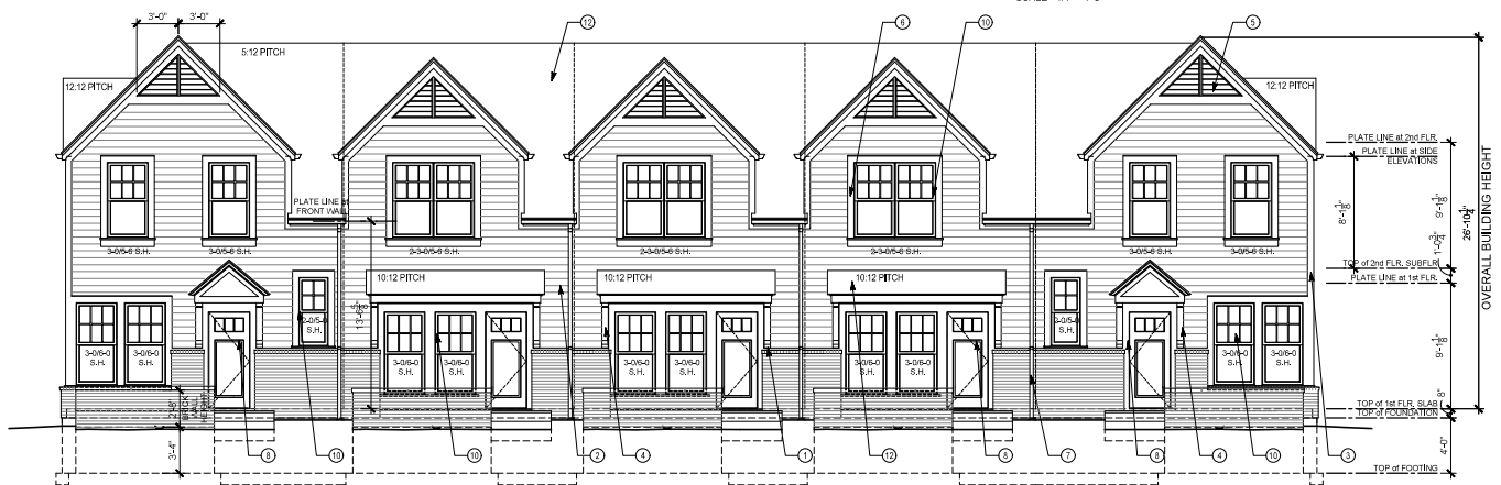
UNIT 11 - A END PLAN UNIT 10 - C PLAN UNIT 9 - C PLAN UNIT 8 - C PLAN UNIT 7 - A END PLAN FRONT - NORTH ELEVATION SCALE - 1/4" = 1'-0"
