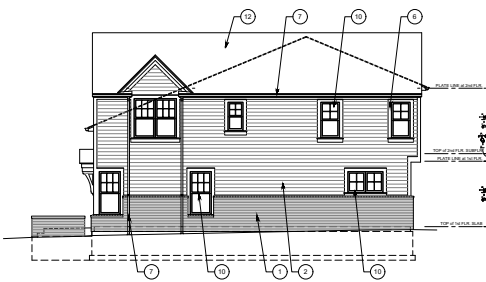
6-UNIT BUILDING SIDE ELEVATION SCALE 1/8" = 1'-0" UNITS 12-17
