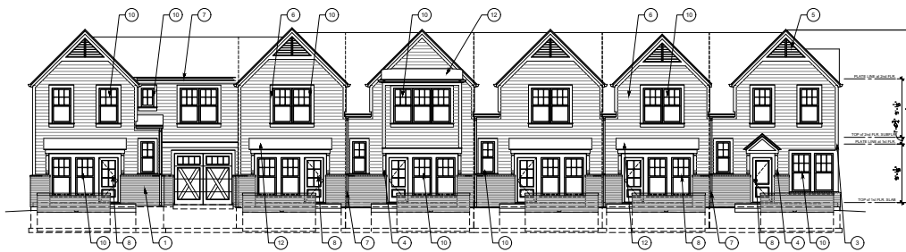
6-UNIT BUILDING FRONT ELEVATION SCALE 1/8" = 1'-0"
