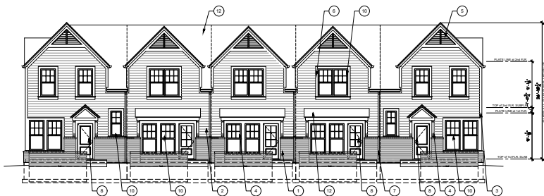
5-UNIT BUILDING FRONT ELEVATION SCALE 1/8" = 1'-0" UNITS 7-11 A UNITS - 2 C UNITS - 3 TOTAL BUILDING AREA 7,776 SQ. FT.
